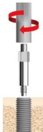
2. The hand-held probe stimulates the SmartPeg magnetically, without actually being connected to it – or even touching it.
